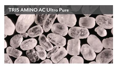
Larger size + fewer fine particles + smoother surface = less clumping. The unique morphology of TRIS AMINO AC buffers helps reduce cake strength, resulting in less clumping and hardness. (4x magnification)
